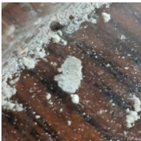
**Figure 9.** Brittle and Fragile film of extracted polymer.
