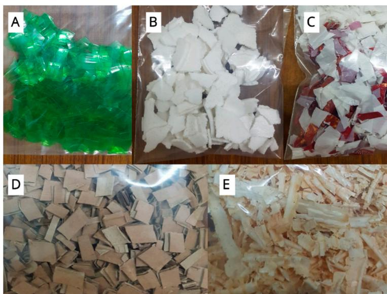
**Figure 10.** Photographs of carbon sources used for optimization of PHA production. (A) Plastic cutouts of a plastic bottle, (B) shredded waste polystyrene cups, (C) shredded plastic bag, (D) cardboard carton cutouts, (E) wood chips.
