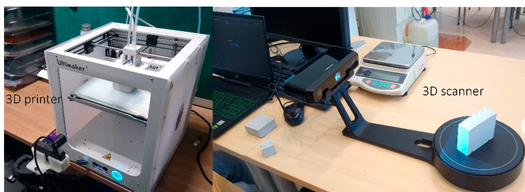
Figure 5. Experimental setup. (Left): 3D printer with infrared camera placed before. (Right): 3D scanner with the object on it.
