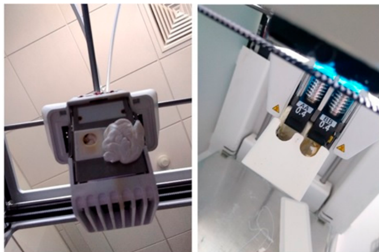
Figure 3. Printer's nozzle damaged by a filament which did not adhere due to warping.
