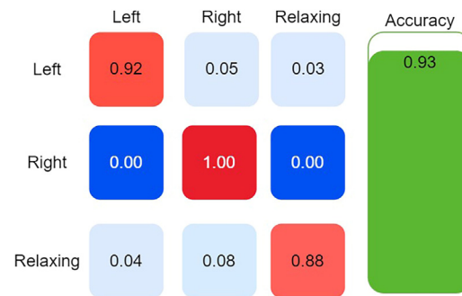
Figure 1. Confusion matrix for real-time three-class classification results for one of the subjects
