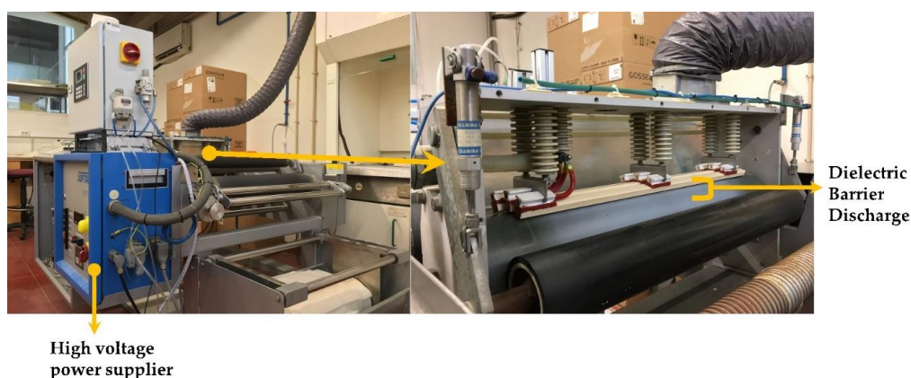
Figure A1. Schematic diagram with a photo of the DBD plasma equipment used for the sample treatment.
