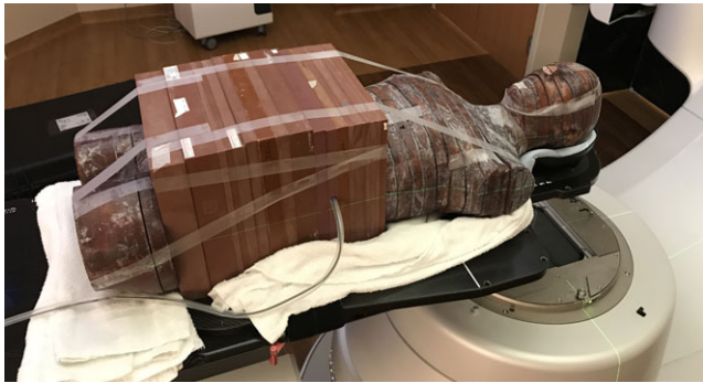
FIG. 2. Modified anthropomorphic phantom used to measure peripheral dose for the candidate treatment plans. Photo shows placement of the ionization chamber approximately at the level of the patient's umbilicus.
