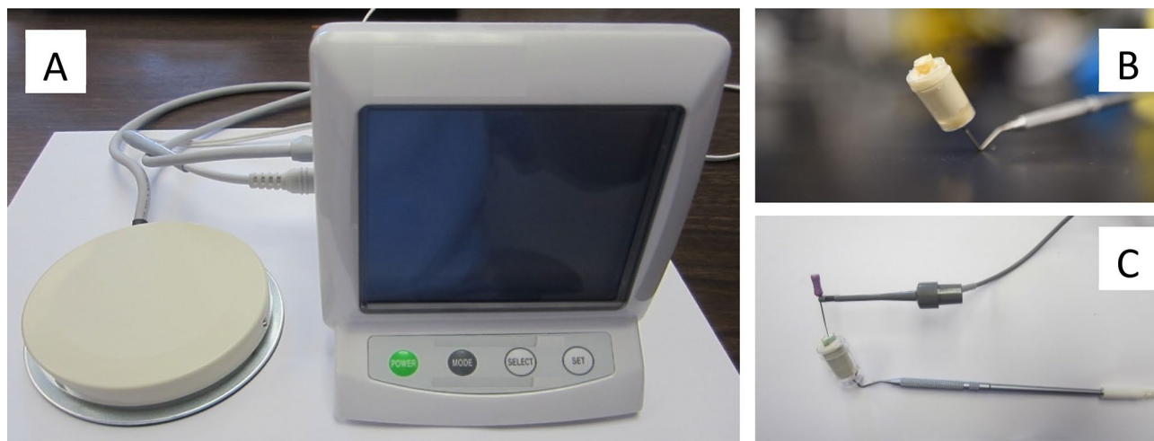
Figure 2. (A) represents the prototype used in the study. For circuit completion, a hole was bored in the inferior portion of the cap to allow the counter electrode, a modified periodontal probe, to be inserted (B). The specimen was mounted in alginate, leaving approximately 2 mm of tooth structure above the alginate (B). The active electrode was created by connecting an insulated #10 endodontic hand file to the device (C).
