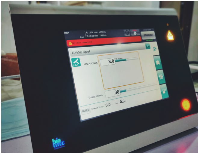
Fig. 2. Leonardo Dual 45 diode laser (Biolitec AG, Jena, Germany); dual wavelength of 980 and 1,470 nm.
