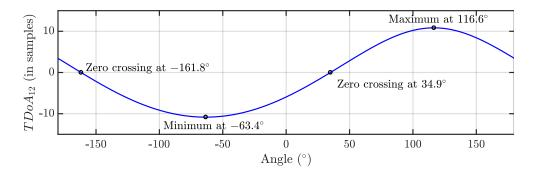
**Figure 3.** Periodic function representing the TDOA vs. the rotating angle. The zero-crossings correspond to the positions of the rig perpendicular to bearing of the source so the distances from the antennas to the source are the same. The maximum and minimum correspond to positions where the rig is parallel to this bearing so one of the antennas is at the farthest relative position with respect to the source and the other at the closest one.
