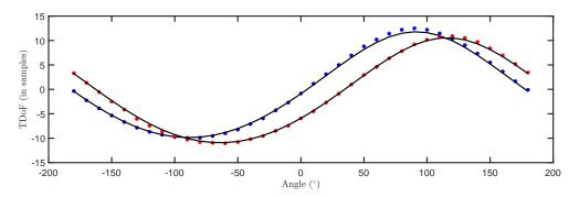
**Figure 16.** Median of all TDOA versus rotation angle in 3D localization with the fitting function. Blue plot corresponds to the fitting function for source 1 and red plot to source 2.
