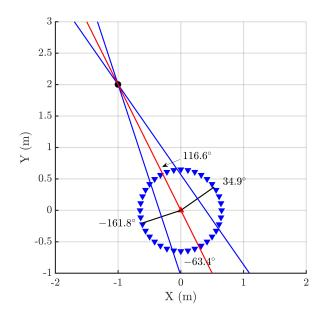
**Figure 1.** Different positions representative of antenna 2 marked with triangles ( $\mathbf{V}$ ) when turned around the fixed antenna 1 ( $\mathbf{A}$ ).
