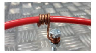
Figure 4. Detail of the section of the high voltage cable (in red) with the wound wire to ground.
