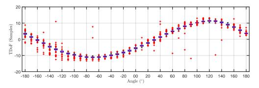
**Figure 15.** Box plot of the time differences of arrival versus angle of rotation for the pulses generated by source 2 in 3D localization.
