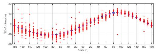
**Figure 9.** Box plot of the time differences of arrival versus angle of rotation for the pulses generated by source 1 (black cluster).
