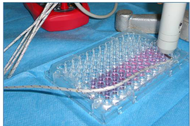
Figure 2. Laser irradiation procedure and measuring the temperature in the wells.
