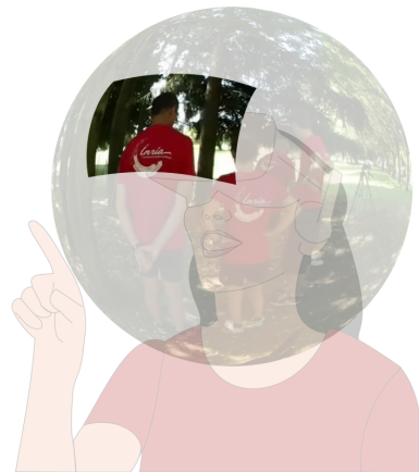
Figure 5. In many applications, including AR/VR/XR and 360-degree video, users are interested in watching a part of a scene (non-shaded area) known as viewport and can freely navigate in the scene enjoying an up to a 6 degree of freedom (DoF) experience.
