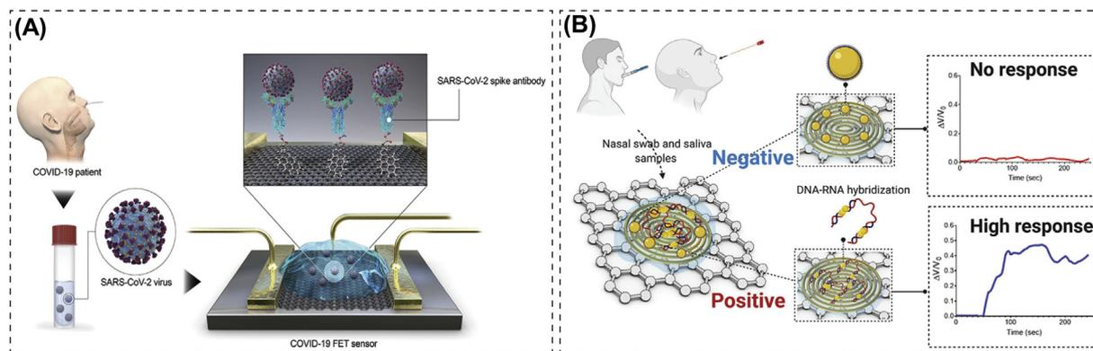
**Fig. 4.** (A) The illustration of the detection of SARS-CoV-2 via FET nanobiosensors with graphene transducers modified with an antibody specific for the SARS-CoV-2 spike protein (Reprinted with permission from Ref. [54]); (B) The illustration of the rapid detection of SARS-CoV-2 viral RNA using an electrochemical sensor made of graphene and gold nanoparticles modified with antisense oligonucleotides (Reprinted with permission from Ref. [56]).
