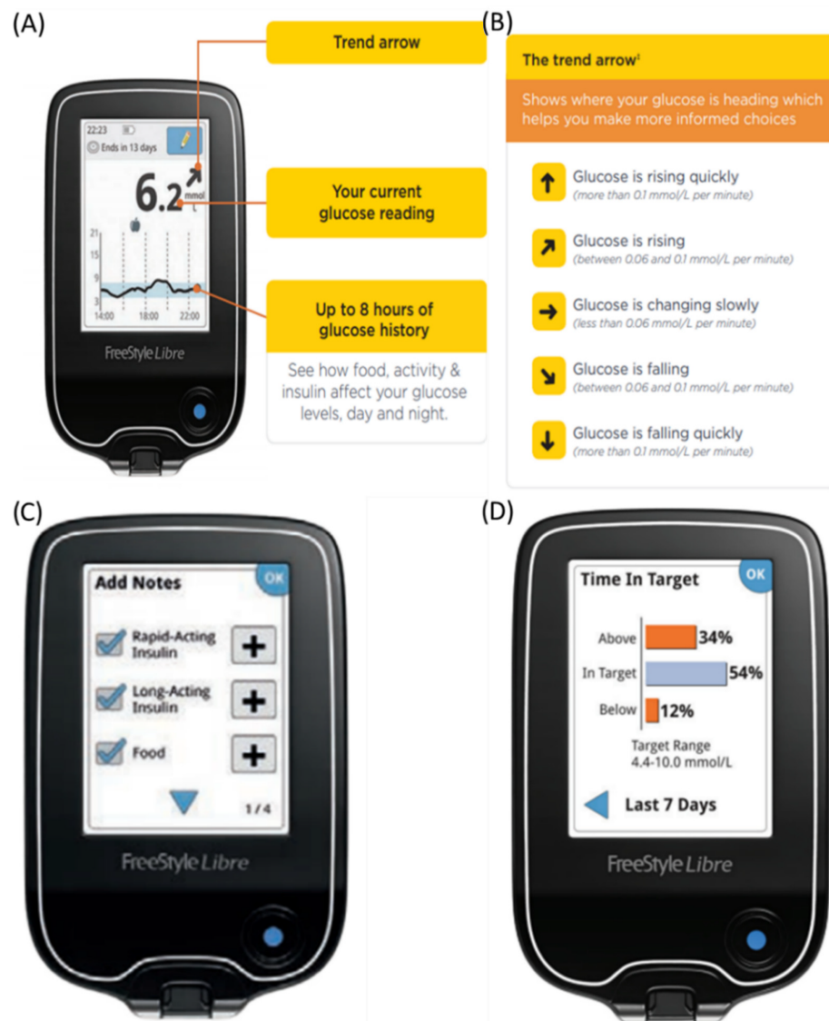
Figure 3. (A) General display of rtCGM indicating the predicted direction of glucose level as shown by the trend arrow, the current glucose reading and eight hours glucose history graph; (B) Description of the trend arrows; (C) Display option of adding notes at a specific time; (D) History of glucose levels based on time in targeted ranges.
