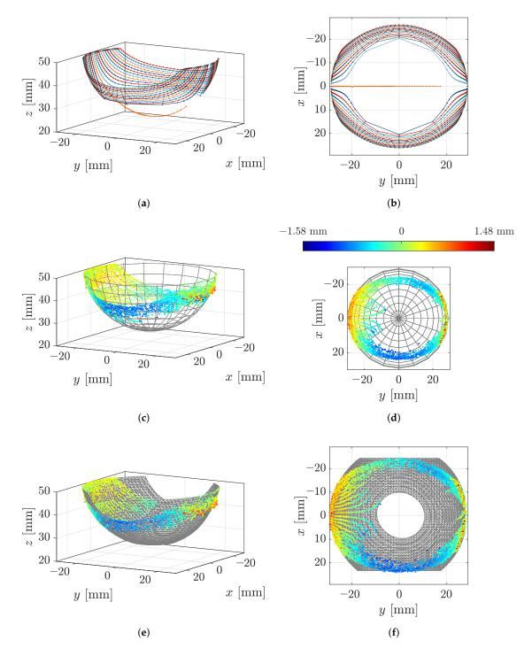
Figure 12. Object reconstruction: (a,b) reconstructed contact points based on simulated data (each connected sequence of points results from one scanning sweep); (c,d) reconstructed contact points based on experimental data superimposed with the original object shape (the color of each point indicates the reconstruction error); (e,f) fitted surface providing a tactile image based on the reconstructed contact points and the corresponding force directions.
