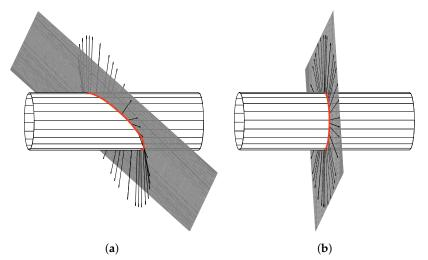
**Figure 3.** Intersection curve (red) between an exemplarily scanned object (cylinder) and the plane of rotation/translation (scanning plane-gray) of the rod: (a) arbitrary arrangement; (b) special arrangement resulting in a plane scanning sweep.
