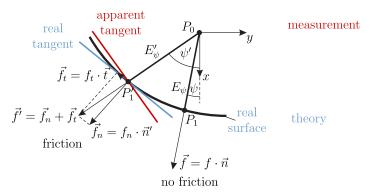
**Figure 13.** Schematic representation of two deformation states at the same clamping position  $P_0$  where one is affected by friction and the other one is the reference state without friction. In the presence of friction, the quantities are marked with an apostrophe— $\vec{f}_t$  is the tangential force component with the magnitude  $f_t$  and direction  $\vec{t}$ ,  $\vec{f}_n$  is the normal force component with the magnitude  $f_n$  and direction  $\vec{n}'$ .
