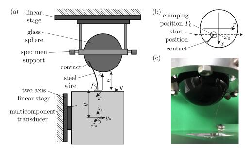
**Figure 6.** Experimental setup: (a) schematic representation of the experiment; (b) top view on (a); (c) one-sided clamped wire in tangential contact with a glass sphere.
