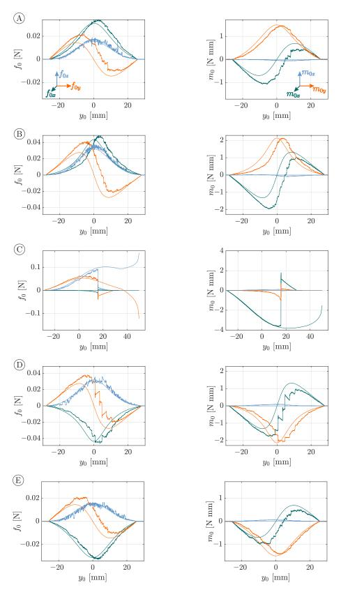
**Figure 9.** Simulated and measured observables, represented by smooth and noisy data, respectively, during object scanning of a 60 mm glass sphere. Each row results from object scanning according to the scanning sweeps (**A–E**), schematically shown in Figure 7, and includes the following diagrams: reaction forces on the left and reaction moments on the right.
