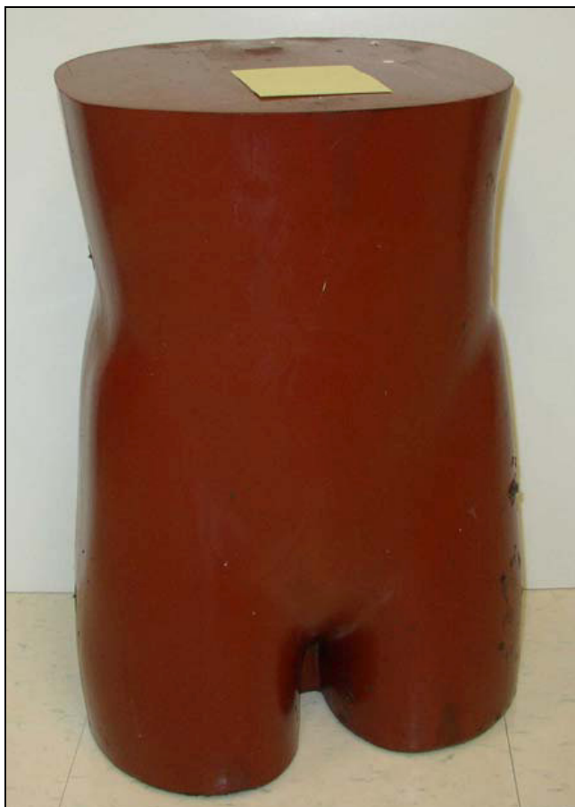
Figure 1 Humanoid abdominal/pelvic phantom.
