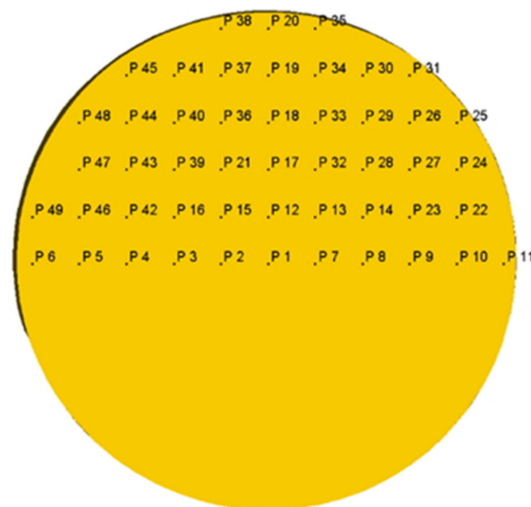
Figure 5. Points in the cross-section of the billet at the stationary stage of screw rolling for which the strain effective values were calculated due to computer simulation.
