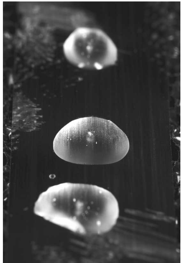
Fig. (1). Plant shoot tips (1 mm diameter) were immersed in droplets of PVS2 cryoprotectant solution on a foil strip, cooled to -196°C and photographed. Transparent nature of droplet suggests that ice did not form during the cooling process. Photo courtesy of Stephen Ausmus, USDA-ARS.
