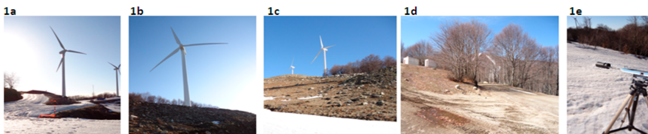
Figure 1. Pictures of the recording positions at: (a) 150 m; (b) 200 m; (c) 1500 m; (d) >2500 m. In (e) is shown the calibration of the sound level meter in situ .
