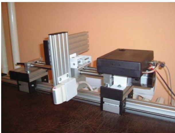
Figure 1. Positioning mechanism of the ultrasound probe.
