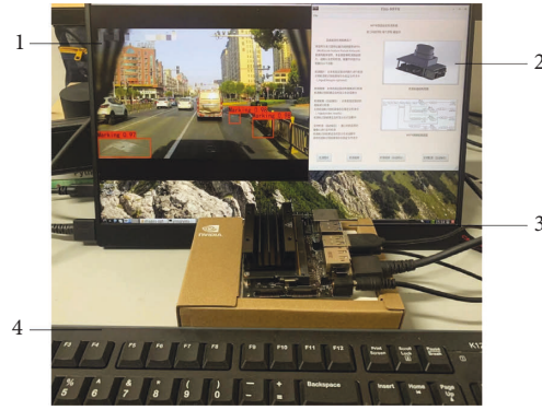
FIGURE 11: Jetson Nano test chart. 1. Test results; 2. Running interface; 3. Jetson Nano; 4. External keyboard.
