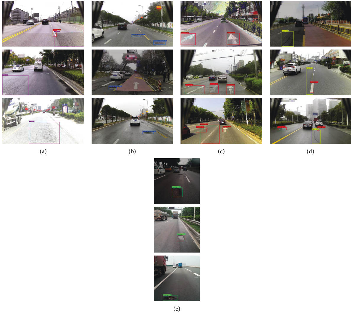
FIGURE 12: Detect results. (a) Net. (b) Manhole. (c) Marking. (d) Crack. (e) Pothole.
