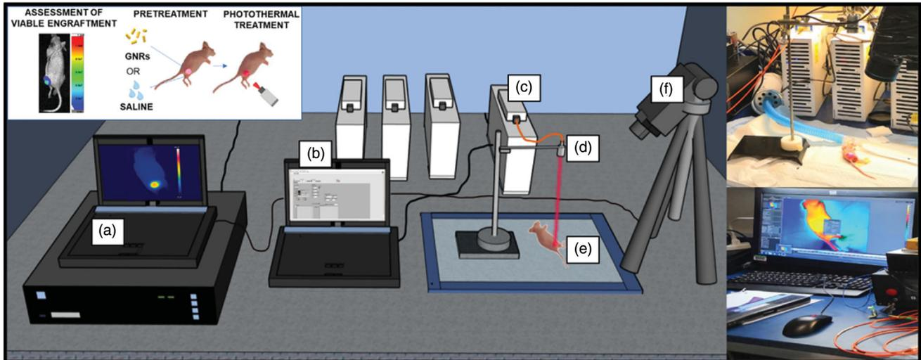
**Figure 3.** Experimental set-up to perform *in vivo* photothermal treatments on breast cancer tumors engrafted on mice flanks. It includes: (a) the computer for monitoring the temperature outcome, (b) the laser software for controlling the laser setting parameters, (c) the NIR laser emitter, (d) the collimator placed at applicator tip, (e) the anesthetized mouse bearing the breast cancer tumor, (f) the thermographic camera adopted for the measurement of the superficial temperatures.
