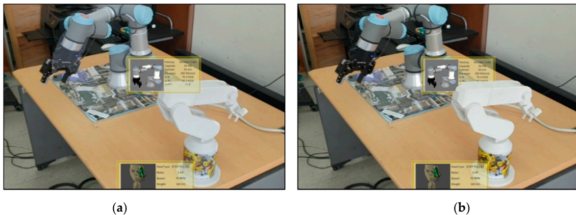
Figure 14. Handling incorrect occlusion during the robot's operation with the proposed approach: AR information can be displayed in a depth perception way: (a) a conventional AR visualization; (b) the proposed AR visualization
