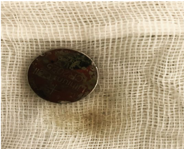
FIGURE 4 A CR2025 battery is a non-rechargeable lithium coin or “button” cell that is 20 mm in diameter and 2.5 mm in thickness.
