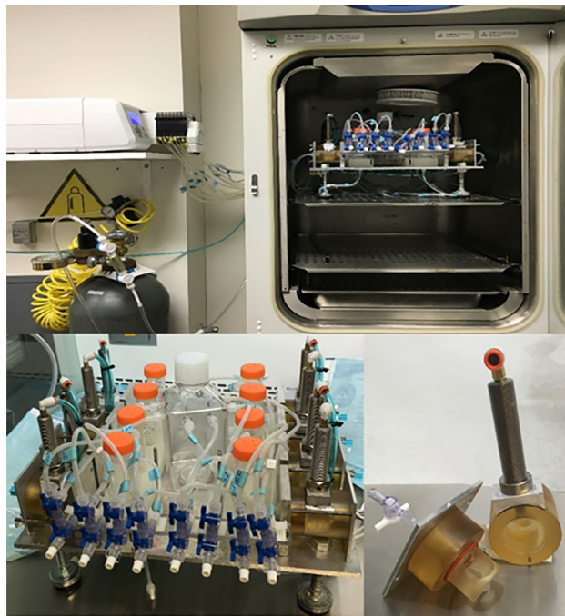
Figure 1. Ex-vivo bone bioreactor setup.
