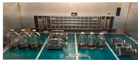
Fig. 1. Experimental setup. 120 mL or 250 mL serum flasks, filling volume 55 mL, shaking frequency 125 rpm, standing or lying.
