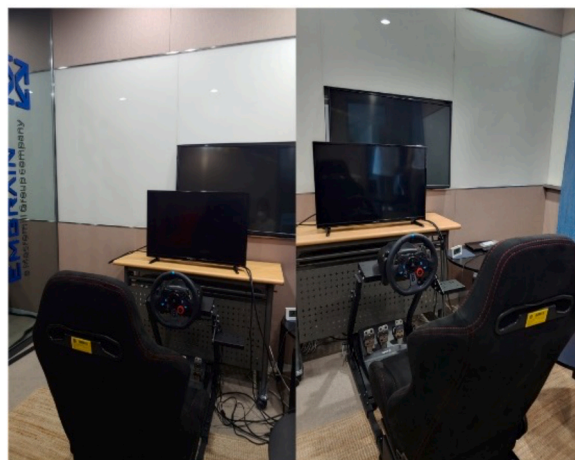
Fig. 9. Laboratory Setting for the Auto-driving Test. A steering wheel and pedals are connected to a PC and Monitor.
