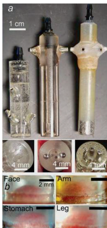
FIGURE 11: Suction electrodes (cited from [65], Figure 1).
