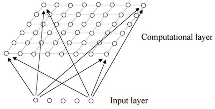
Fig 1. Two dimensional SOM neural network model.
