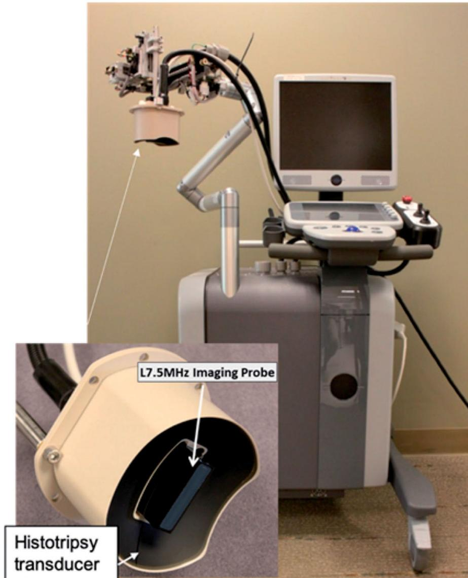
**Figure 4.** An ultrasound-guided histotripsy system that contains an ultrasound imaging engine, a histotripsy transducer with the imaging probe in the center (insert), a positioning arm that mechanically moves the histotripsy transducer.
