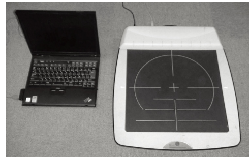
Fig. 1. Win-pod (MEDICAPTEURS). Win-pod consists of a computer, a sensor plate, and a display monitor and it is used for podometry data analysis such as multi steps acquisition, analysis per foot area, static and dynamic analysis.
