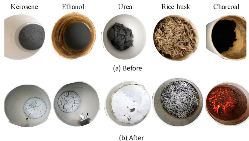
Figure 4. Appearances of the mixed fuel agent and raw materials (micro-silica and \text{CaCO}_3 powders) before and after calcination.
