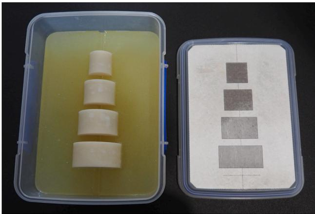
**Fig. 4.** One set of vertebrae installed in soft-tissue analogue. The lid is attached after the dry rice is poured into the container; the dashed lines on the lid label form a target for precise alignment of the vertebrae with the cross-hairs of the DXA scanner.
