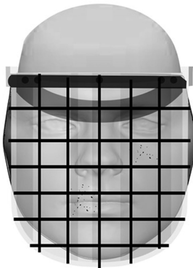
FIGURE 4 The face shield contained a grid pattern. In the simulated case illustrated, the sample run would score a three because three squares contain spatter
