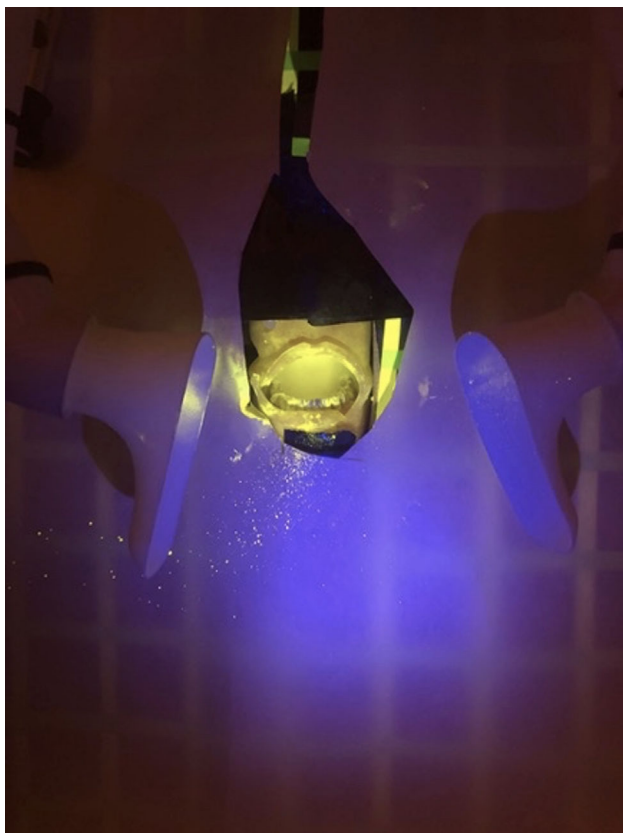
FIGURE 3 Fluorescence Spatter after a test run. Grid is covered with new paper prior to each test run
