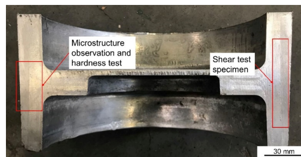
Figure 7. Physical diagram of cross-section of the brake drum and its sampling position and function.
