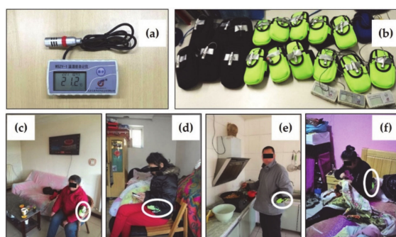
Figure 2. Personal experienced temperature monitoring devices. (a) Temperature logger and (b) devices used for monitoring. The three on the lower right were not placed in armband sleeves. (c) A volunteer wearing a device and sitting in the living room while watching TV. (d) A volunteer wearing a device and sitting in the bedroom playing with her smartphone. (e) A volunteer wearing a device and standing in the kitchen to cook. (f) A volunteer wearing a device and sitting in the bedroom to sew a quilt. The monitoring devices in (c–f) are circled with white ovals.
