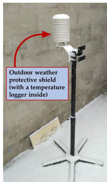
Figure A1. An outdoor air dry-bulb temperature logger with protection installed in household A#1.
