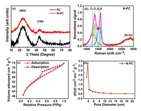
**Figure 4.** (**a**) XRD pattern and (**b**) Raman spectrum of N-PC with a deconvolution of the D/G spectral region (**c**) nitrogen adsorption/desorption isotherm and (**d**) Barret–Joyner–Halenda model (BJH) pore size distribution plot of N-PC.
