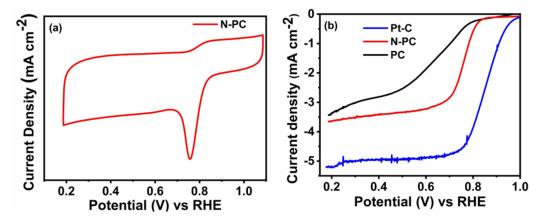
**Figure 6.** (a) CV curves of N-PC in  $O_2$  saturated; (b) LSV curves of PC, N-PC and Pt-C obtained from the RRDE measurement with rotating speed of 1600 rpm in 0.1 M KOH at a scan rate of 10 mV s<sup>-1</sup>.
