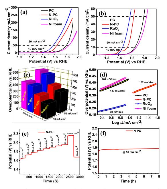
**Figure 8.** (**a**,**b**) Oxygen evolution reaction (OER)-LSV curves of PC@Ni, N-PC@Ni, RuO<sub>2</sub>@Ni and Ni foam in 1 M KOH at a scan rate 1 mV s<sup>-1</sup> [with iR-correction]; (**c**) bar of prepared catalyst vs overpotential at 10 and 50 mA cm<sup>-2</sup>; (**d**) Tafel slopes of PC@Ni, N-PC@Ni, RuO<sub>2</sub>@Ni and Ni foam; (**e**) multiple-step chronopotentiometric of N-PC@Ni; (**f**) chronopotentiometric curve of N-PC@Ni at a constant of 50 mA cm<sup>-2</sup>.
