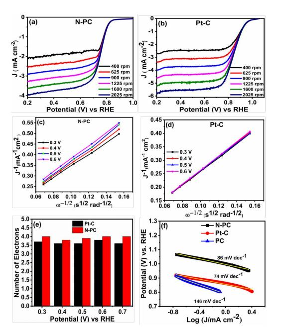
**Figure 7.** LSV curves of (**a**) N-PC and (**b**) Pt-C obtained from RRDE measurement with different rotation speeds in  $O_2$  saturated 0.1 M KOH at a scan rate of 10 mV s<sup>-1</sup>; Koutecky–Levich plots of (**c**) N-PC (**d**) Pt-C; (**e**) plot of potential vs number of electrons and (**f**) Tafel slopes of PC, N-PC and Pt-C.
