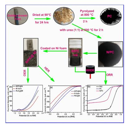
**Figure 1.** Schematic representation of the synthesis of N-doped porous carbon (N-PC) from golden shower pods biomass (GSB) and its electrochemical activity. (Abbreviations: porous carbon (PC), N-doped porous carbon (N-PC), ring rotating disc electrode (RRDE), oxygen evolution reaction (OER), hydrogen evolution reaction (HER) and oxygen reduction reaction (ORR)).
