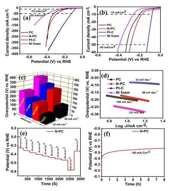
**Figure 9.** (**a**,**b**) Hydrogen evolution reaction (HER)-LSV curve of PC@Ni, N-PC@Ni, Pt-C@Ni, and Ni foam in 1 M KOH solution at a scan rate 1 mV s<sup>-1</sup> [with iR-correction]; (**c**) bar of prepared catalyst vs overpotential at 10 and 50 mA cm<sup>-2</sup>; (**d**) Tafel slopes of PC@Ni, N-PC@Ni, Pt-C@Ni and Ni foam; (**e**) multiple-step chronopotentiometric of N-PC@Ni; (**f**) chronopotentiometric curve of N-PC@Ni at a constant of  $-50 \text{ mA cm}^{-2}$ .
