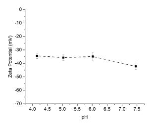
**Figure 2.** Zeta potential titration for Fe<sub>3</sub>O<sub>4</sub>@SiκCRG particles.
