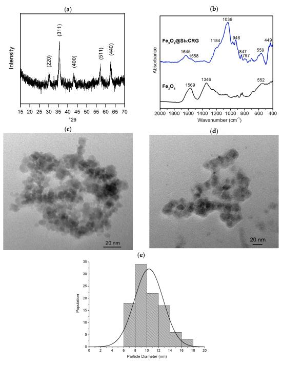
**Figure 1.** Physicochemical characterization of nanoparticles. (a) XRD diffraction pattern, with Bragg reflections identified. (b) ATR-FTIR spectra, with main bands identified. TEM images of  $Fe_3O_4$  (c) and  $Fe_3O_4$ @SikCRG (d) nanoparticles. (e) Histogram for size distribution of  $Fe_3O_4$  core nanoparticles.
