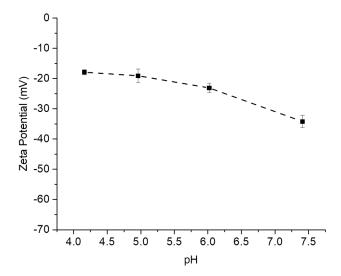
**Figure 5.** Zeta potential titration for  $Fe_3O_4@Si\kappa CRG$  particles loaded with doxorubicin (loading capacity was 3.2 wt.%).
