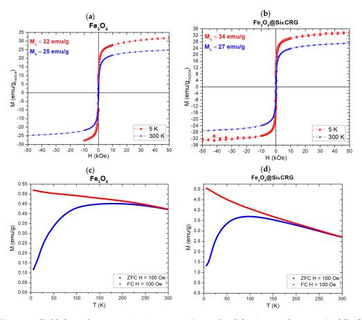
**Figure 3.** Field dependent magnetization curves (normalized for iron oxide content) of  $Fe_3O_4$  nanoparticles (a) and  $Fe_3O_4$ @SikCRG nanoparticles (b). Temperature dependent magnetization curves of  $Fe_3O_4$  nanoparticles (c) and  $Fe_3O_4$ @SikCRG nanoparticles (d).
