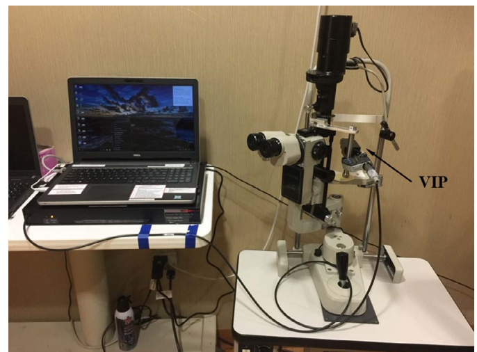
Figure 2. Photograph of the VIP system in the clinical setting. The VIP head is mounted onto a standard slit lamp.
