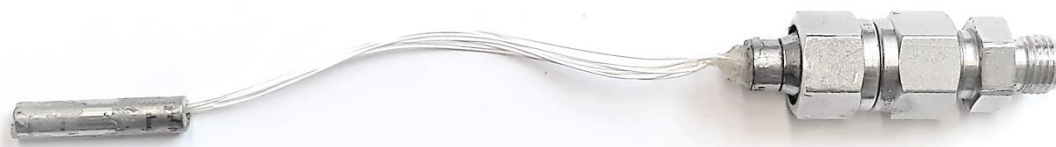
Figure 1. The membrane module containing the polyimide capillaries.
