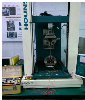
Figure 4. Experimental setup of the tensile test.
