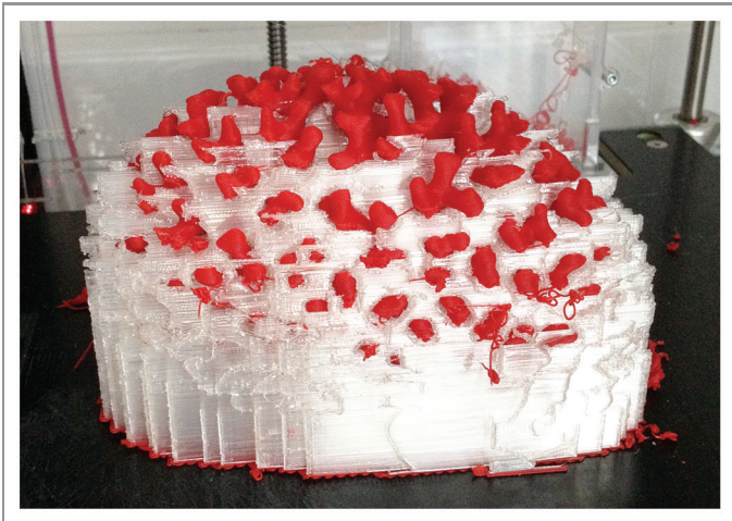
Figure 2. Branching ureteric tree from an E15.5 mouse kidney printed in red ABS plastic, demonstrating the extensive white PLA support scaffold required.
