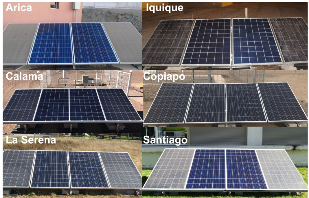
Figure 2. Photographs of the soiling measuring systems. At each location, the central modules of the arrays were manually cleaned while we allowed the other two to naturally accumulate soiling. Please note that these pictures were not taken at the same time and they are not meant to show the typical soiling, since the latter significantly changes during the year. Photographs were taken by the authors (R.R.C., J.J., E.S., D.S., and S.M.).
