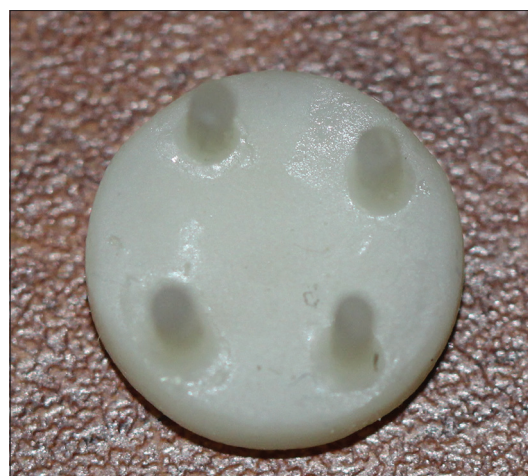
Figure 1: Specimen fabrication with resin cement cylinders on lithium disilicate discs
