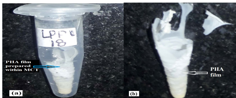
Fig. 8 a PHA film for Bacillus sp. LPPI-18 after treated with SDS-NaClO solution and dissolved within chloroform using microcentrifuge (MCT) as molding material. b A partly fractured PHA film after it had dried and was removed from MCT
