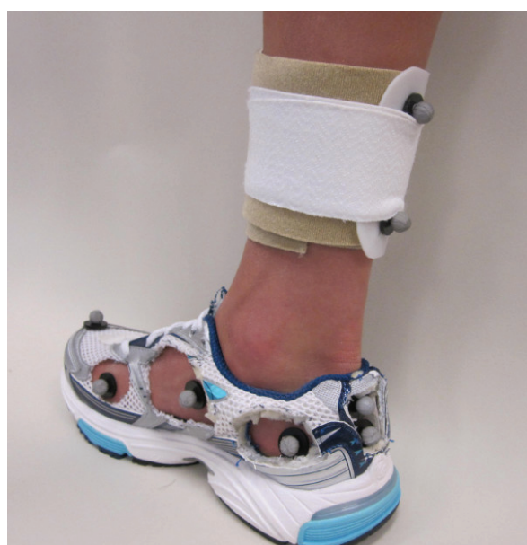
Figure 3 Marker set-up for kinematic data collection.
