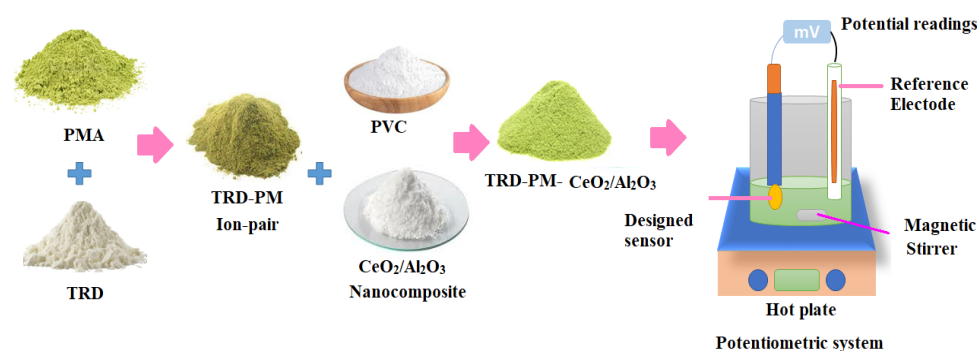
Figure 2. Preparation of TRD-PM-CeO 2 /Al 2 O 3 electroactive complex and the potentiometric system employed for TRD determination.
