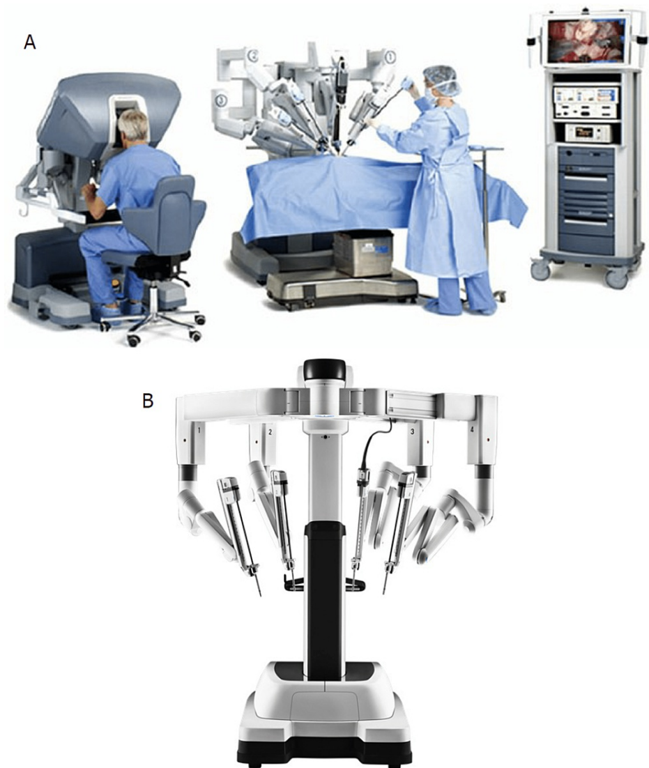
FIGURE 1: Model of the Da Vinci Surgical System having three major components: (1) the surgeon's console; (2) a surgical cart with the robotic arms and end-effectors; and (3) the visual cart.
