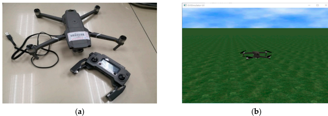
Figure 6. Semi-physical simulation system: (a) Physical part of the simulation; (b) Screenshot of the software.
