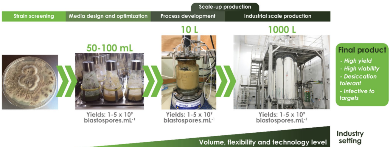
Fig. 6 Submerged liquid fermentation of filamentous entomopathogenic fungi: from small- to large-scale production. In this example, a biotechnological platform supporting cost-effective high yields of viable and desiccation-tolerant blastospores has been implemented after several years of research, including a cutting-edge patent tech-
