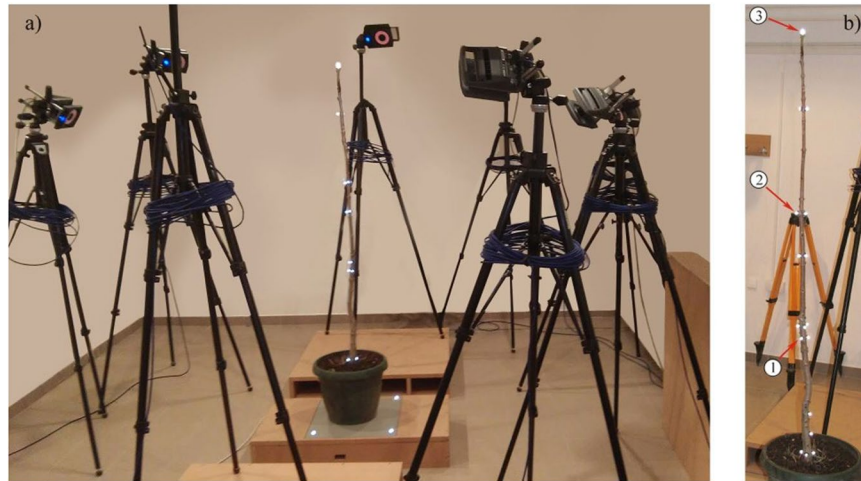
Figure 1. (a) The Vicon 3D motion capture system; (b) A tree under considerations with several markers along it and three markers numbered (1, 2 and 3).
