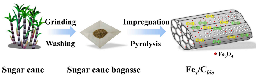
Scheme 1. The synthesis procedure of Fe x /C bio catalysts
